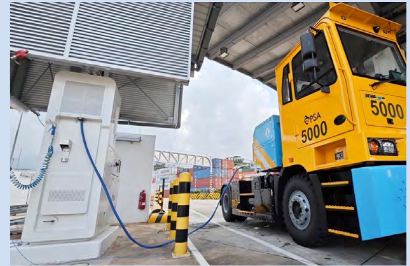
Hydrogen fuel cell electric prime mover at Pasir Panjang Terminal (photo credit: PSA Singapore)
