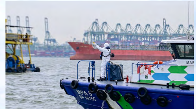
MPA chemical site team measured methanol concentration in the air to mark out "hot" and "warm" zones
